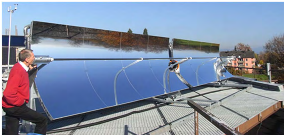
NEP PT1800 collector on test site of SPF
